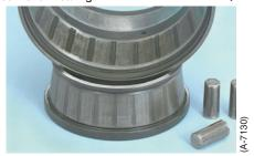
■ Rust on outer ring raceway surface of Tapered Roller Bearing
