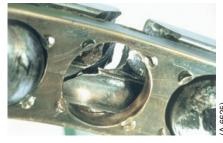
■ Crack in outer ring of Double-Row Cylindrical Roller Bearing
