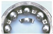
Crack of Tapered Roller Bearing cage
