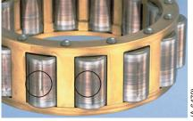
■ Rust on inner and outer rings and on roller of Tapered Roller Bearing Rust on roller pitch of one row.
