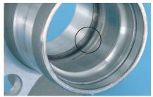
■ Rust on outer ring raceway surface of Double-Row Cylindrical Roller Bearing
