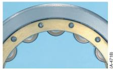
Wear on outer ring raceway surface of Double-Row Cylindrical Roller Bearing
